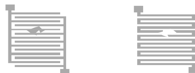
Fig. 1: Basic test structures to detect short circuit (left) and open circuit defects (right)
