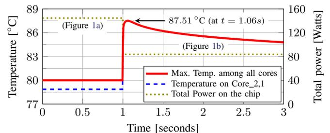
Fig. 2: Motivational example: Transient temperatures. During  $t = [0s, 1s]$  there are 12 active cores according to Figure 1a. During  $t = [1s, 3s]$ , we activate 4 cores according to Figure 1b. The highest transient temperature happens on the core in the 2<sup>nd</sup> row and 1<sup>st</sup> column, that is, Core\_2,1, at  $t = 1.06s$ .
