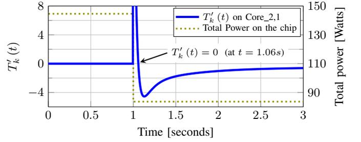
Fig. 3: First-order derivative of the temperature on Core\_2,1 for the transient simulations in Figure 2. After the change in power,  $T'_k(t)$  is zero at  $t = 1.06\text{s}$  and when  $t \rightarrow \infty$ .
